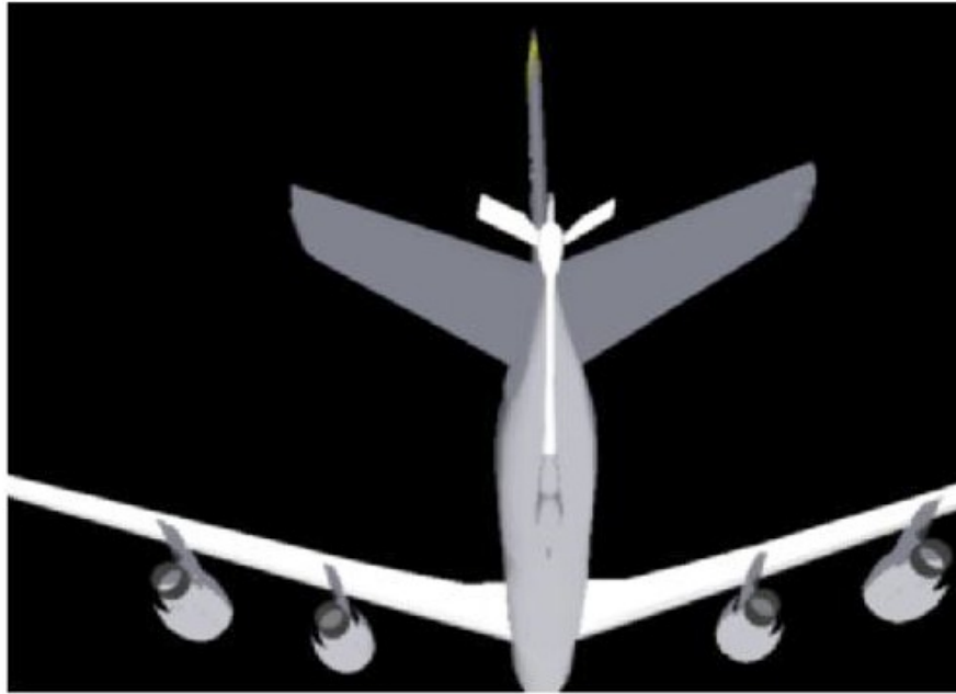
Figure 3: Sample rendering of the KC-135R from the trailing aircraft's perspective. The model is rendered using the Matlab Virtual Reality Toolbox.
